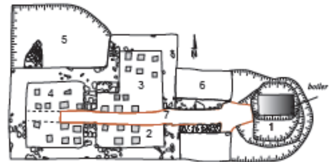
1 - Heating Area 2 - Caldarium (Hot room) 3 - Sauna ? 4 - Tepidarium (Tepid room) 5 - Frigidarium / Apodyterium (Cold room) 6 - Praefurnium (Oven structure) 7 - Heating canal
